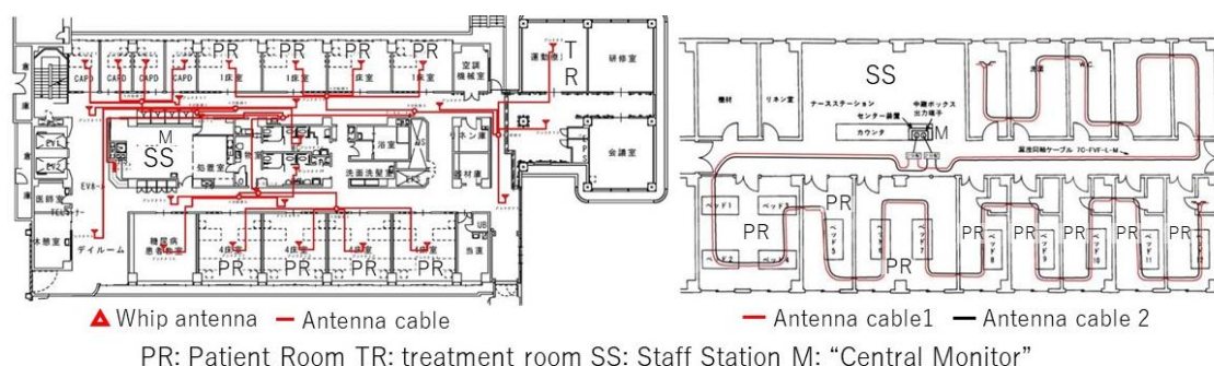
Figure 2. Antenna systems used in Japanese wireless telemetry systems (Left, Multi antenna system: Right, Leaky co-axial cable system)
